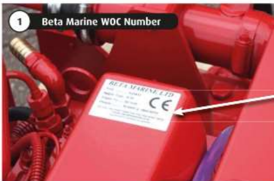
The engine specification label is located on the engine rocker cover, it details the WOC number, engine type, engine serial number and output in bhp.
